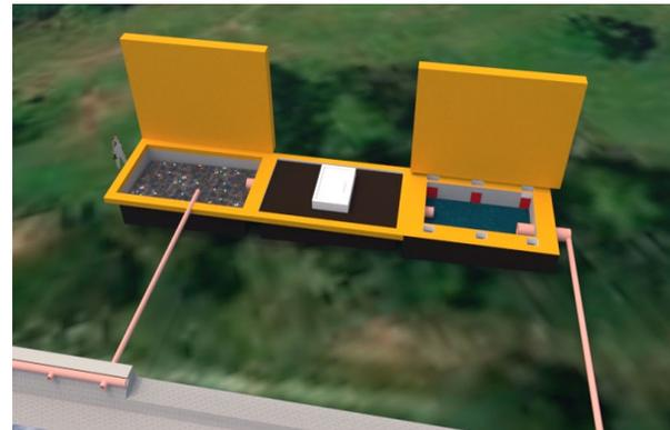
As shown above, the design mainly utilizes concrete hollow blocks, steel and the pipes. As for the hollow blocks, a 6" concrete hollow block shall be used for the main wall of the structure. As for the pipes, standard Polyvinyl Chloride (PVC) Pipes are used both on the piping system upon connecting the pipes into the wastewater UV treatment system.
